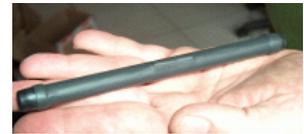
**Long range Stick Ecotags** - Battery assisted (active) stick type transponders with 25 to 30 meter range (5uW sensitivity). Battery life 3 months on continuous use. Cased in hard rubber. (Generally used with the radar reader).
