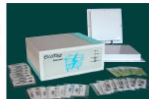
**Small portable system (long range)**- Portable Reader, 100 creditcard sized 200 uW transponders, charger and cables (10 meter range)
